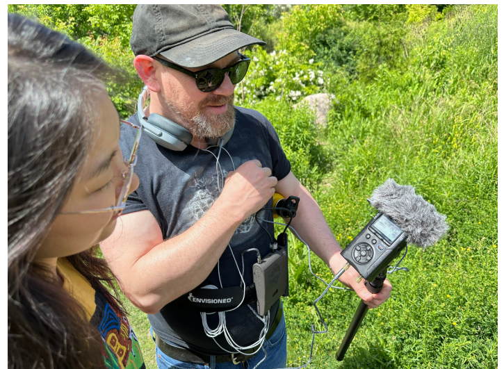
Figure 1. Mark-David Hosale equipped with a Tascam DR-40, on a boom arm, and The Source by bioMECI, worn around the waist, collecting a simultaneous stereo field recording and his own biophysiology. Wen Luo and Mark-David Hosale are shown (from left to right). Image courtesy of Marcus Gordon (a.k.a. magfoto) ©2024 Marcus Gordon
