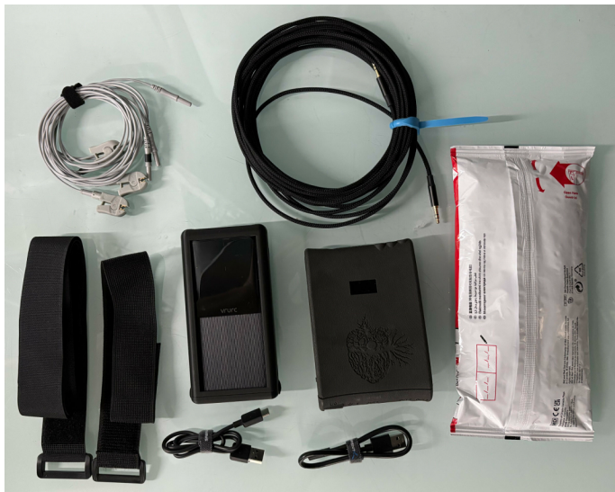
Figure 2. Pictured above are the basic components of the The Source kit. From left to right, top to bottom there are the electrode leads, audio cable, two straps (large and small), the battery pack (with USB-C charging cable, shown below it), The Source (with USB mini connection cable, shown below it), and electrodes. Image: ©2024 bioMECI
